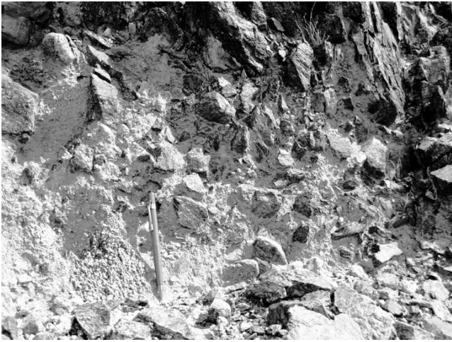
Figure 19. Basal rupture zone exposed at the toe of the southern Alcoholic Pass landslide. Note how matrix-supported angular breccia clasts grade upward to clast-supported breccia.
