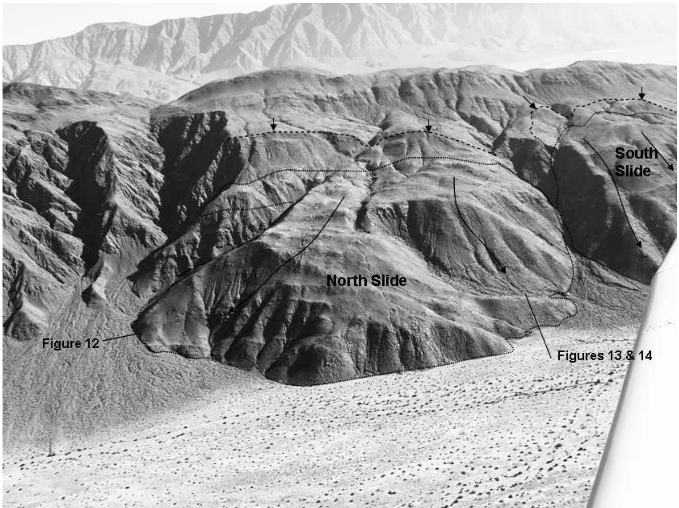
Figure 10. Heavily eroded north slide and portion of south slide, Coyote Peak landslides, showing location of Figures 12, 13, and 14. Short arrows point to top of headscarps. View is to east from Borrego Valley.
