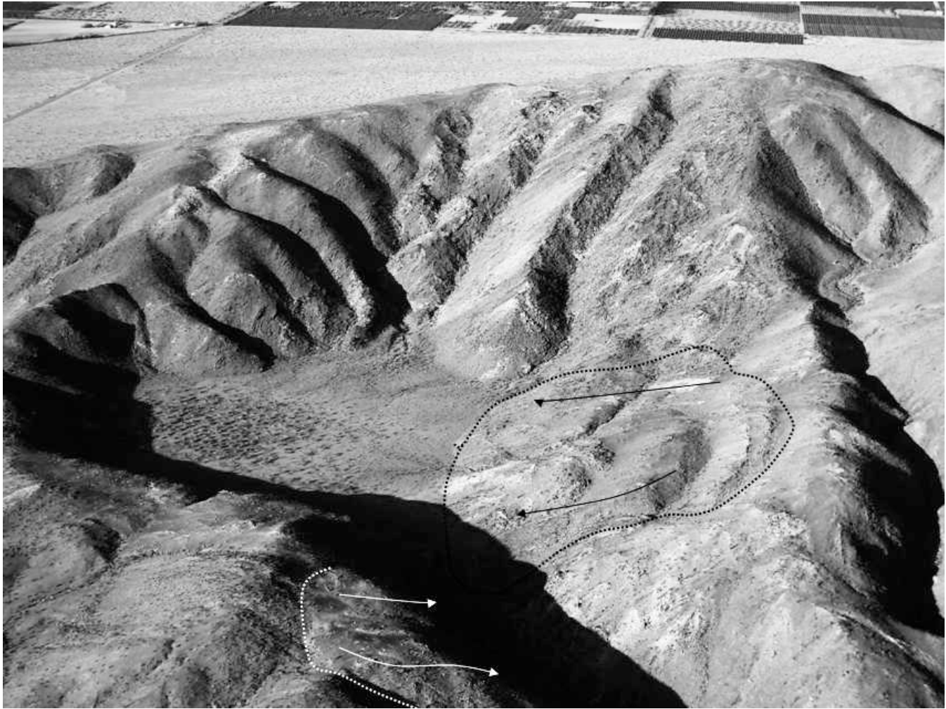
Figure 8. Landslide dam north of the Peg Leg Smith landslide complex. See Figure 6 for location. Trapped alluvium in valley is estimated to be 150 ft (47 m) thick.
