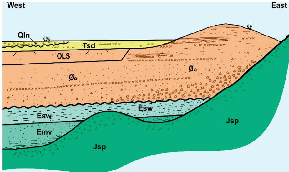
Figure 3. Generalized geologic cross section of southwest San Diego County. Jsp, Santiago Peak Volcanics; Emv, Eocene Mission Valley Formation; Esw, Eocene Sweetwater Formation; Øo, Oligocene Otay Formation; OLS, Otay Mesa Lateral Spread; Tsd, Pliocene–Pleistocene San Diego Formation; Qln, Pleistocene Lindavista Formation. Figure is modified from Walsh and Demere (1991).
