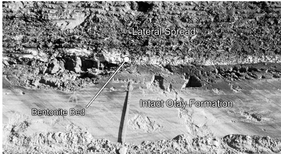
Figure 10. Close-up photograph of the contact between the intact Otay Formation and the Otay Mesa Lateral Spread in Poggi Canyon. The flat-lying bentonite bed is clearly visible. Note the loose unconsolidated appearance of the Otay Mesa Lateral Spread debris. The striations in the lower portion of the photograph were caused by grading equipment.
