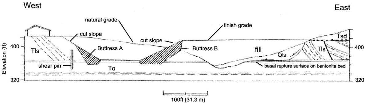
Figure 15. Cross section through a residential subdivision in Chula Vista showing typical buttressing and grading required for stabilization of Otay Mesa Lateral Spread basal rupture surface.
